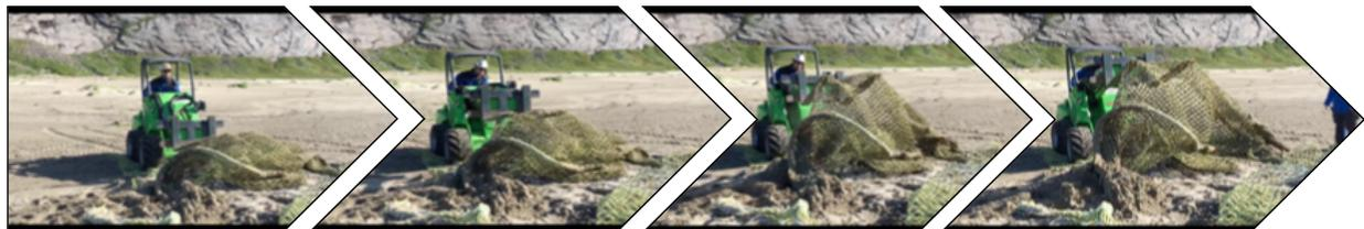
Figure 14: Photo sequence showing how partially buried ALDF was lifted loose from the sand with the forklift. This was done incrementally by repeatedly reattaching the forklift lower down on the net after releasing a section, as well as moving the wheel loader around the mound to dislodge different parts of the net.
