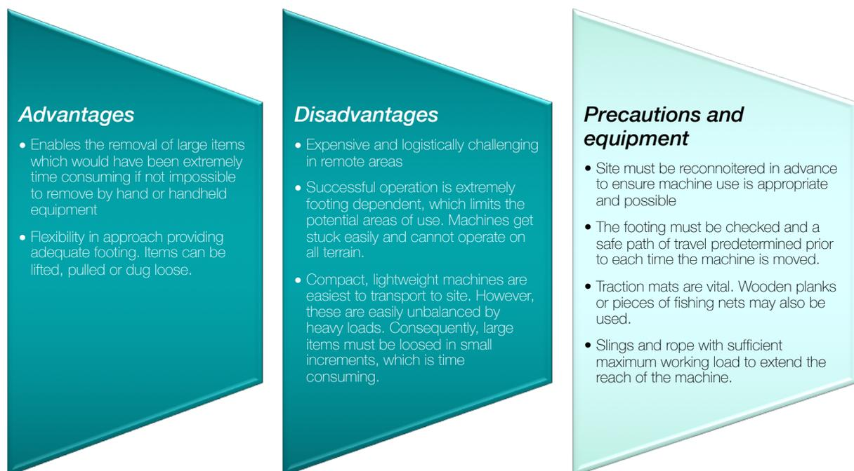
Figure 15: A brief overview of the general advantages and disadvantages of using machinery, as well as some of the necessary precautions and equipment. For comments on differences between machines, see text.
