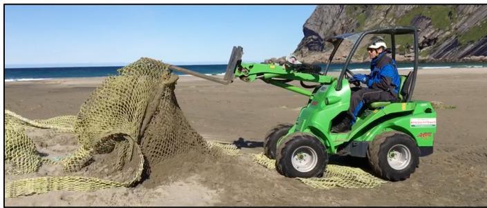
As the wheel loader was equipped with both a bucket and a forklift, we could choose to either dig, lift or pull litter loose from the sand. However, given the sheer size of some ALDF, using the bucket to dig and lift was not practical. Using the wheel loader to pull items loose by tying it to the machine and slowly driving away
