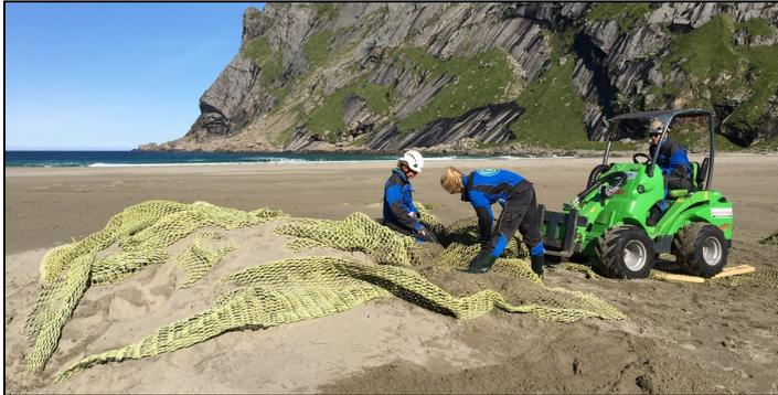
Figure 13: Preventing the wheel loader from getting stuck during operations required fishing net mats to reduce spinning of the wheels (bottom), and most often also wooden planks beneath the wheels (top) to spread the machine's weight and provide a solid surface to drive on. This was increasingly important as the sand around the item being dislodged became disturbed, and to allow the wheel loader to get close enough to the edge of the mound.
