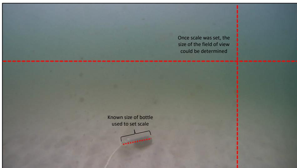
Figure 1: Sample still image from ROV videos showing one of the bottles on the rope transect used to set the scale (i.e. pixels per cm), and subsequently to determine the field of view (area shown in the image, calculated as width x height and given in  $m^2$ ).
